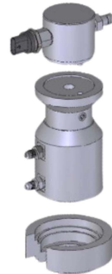
Adapters for injector mounting on cam-box
